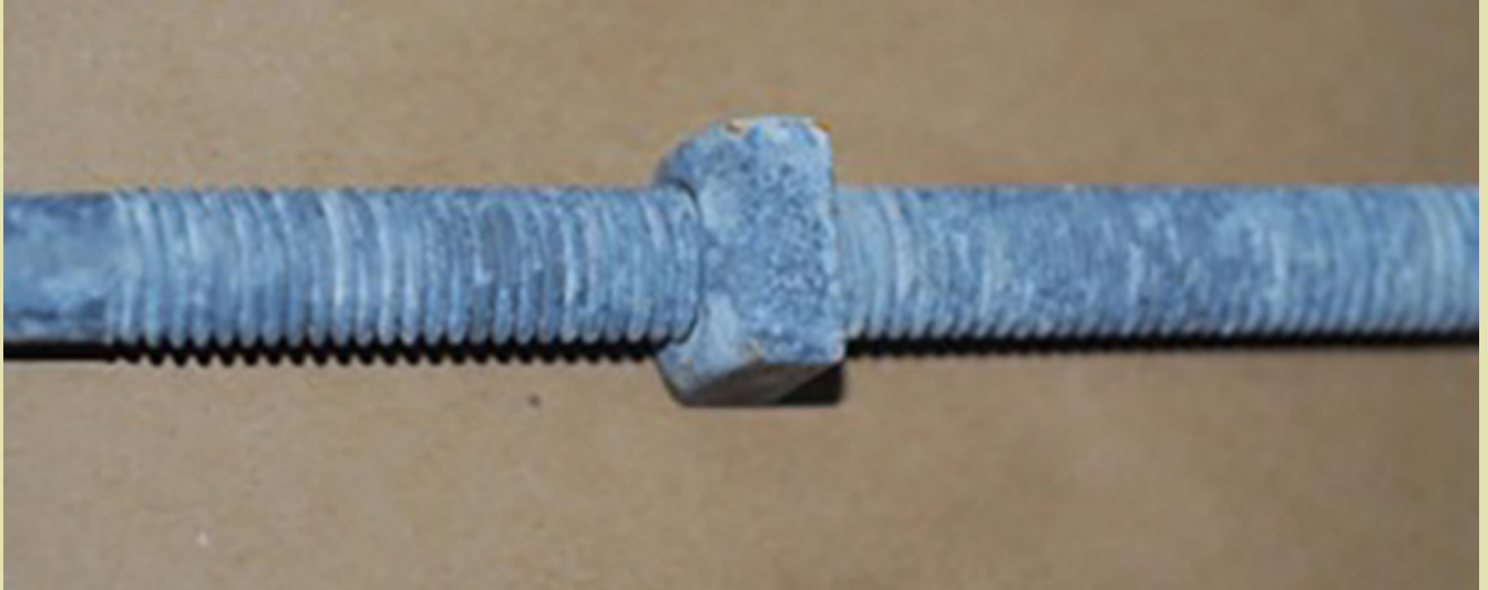
Part No. 75816 5/8" X 16" Square Head Machine Bolt TDG Finish After 504 Hours No Red Rust
