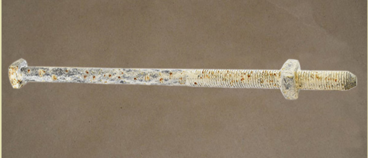
Part No. 8226 5/8" X 14" Square Head Machine Bolt Hot Dip Galvanized After 750 Hours
