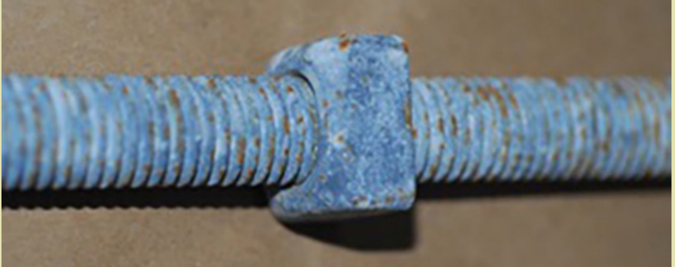
Part No. 75816 5/8" X 16" Square Head Machine Bolt TDG Finish After 2520 Hours Slight Red Rust
