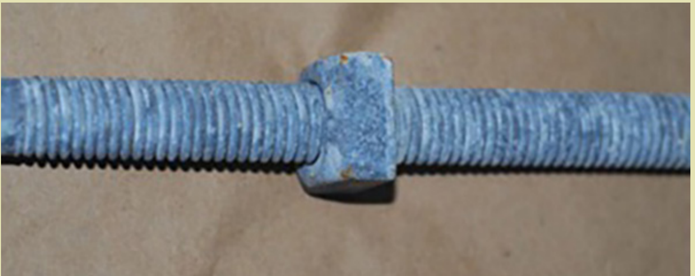
Part No. 75816 5/8" X 16" Square Head Machine Bolt TDG Finish After 1008 Hours Slight Appearance of Red Rust
