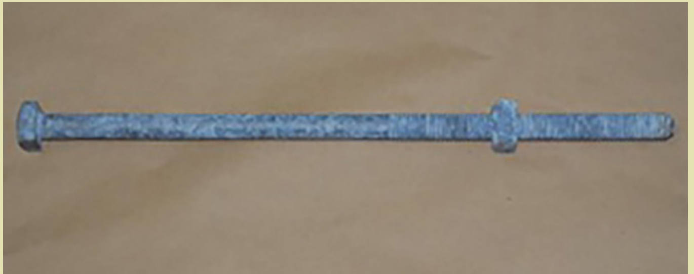
Part No. 75816 5/8" X 16" Square Head Machine Bolt TDG Finish After 504 Hours No Red Rust
