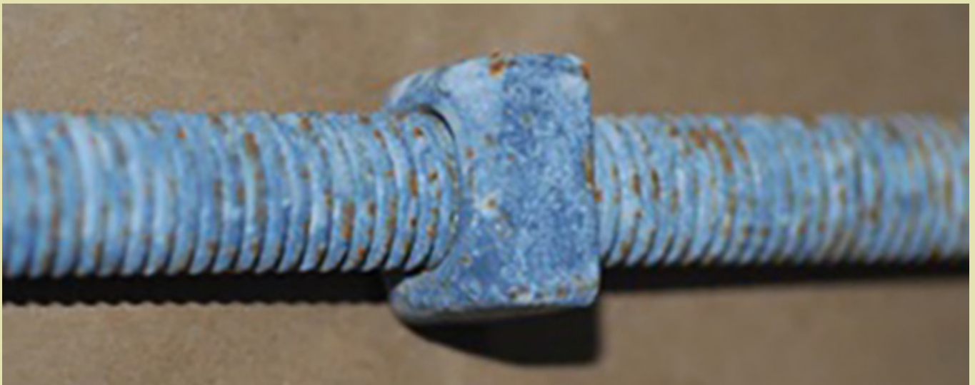
Part No. 75816 5/8" X 16" Square Head Machine Bolt TDG Finish Test Concluded at 2712 Hours Red Rust Beginning to Become More Prevalent
