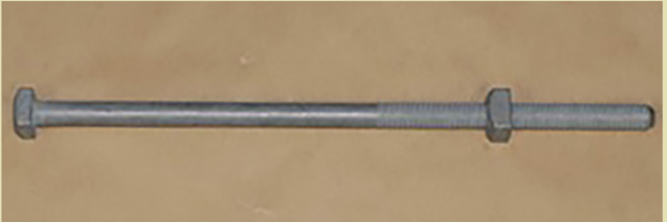
Part No. 75816 5/8" X 16" Square Head Machine Bolt TDG Finish Before Salt Spray Testing Per ASTM B117
