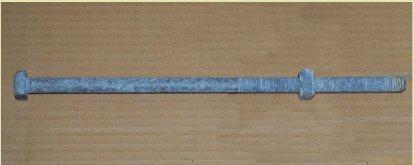
Part No. 75816 5/8" X 16" Square Head Machine Bolt Thermal Diffusion Galvanizing After 750 Hours
