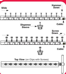
Insert Strip Clips<sup>TM</sup> into dispensing sleeves supplied with each carton. Place clip on cable while still linked together in the dispensing sleeve. Pull cable tight and fasten with nail or drive screw.
