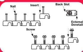
Strip Clips<sup>TM</sup> are preassembled with 12 clips linked together. Additional strips can be snapped together for continuous feed.
